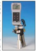
assemble the unit every time you need it. The calibrator (indicator) can at any time be used separately for other pressure test tasks. A special quick connector between the pump and the indicator makes it possible to seperate the system in seconds and to swivel the indicator for easy viewing.
