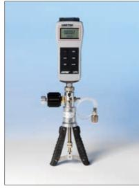
The indicator and the pump are fitted with a special quick connector that makes it possible to seperate the system in seconds without any tool. This quick connector also makes it possible to use the assembled system with the indicator twisted to any angle.
