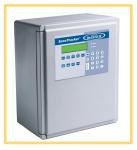
The SonoTracker™ Ultrasonic Level System. The system can monitor up to 16 vessels with transducers of various frequencies, and vessels of different heights and shapes and accurately measure the level of many different materials. It allows you to read levels from 1 foot to beyond 100 feet in solids, and additionally the same unit does open channel flow and differential level measurements.
