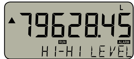
F173 with linearization & backlight off
