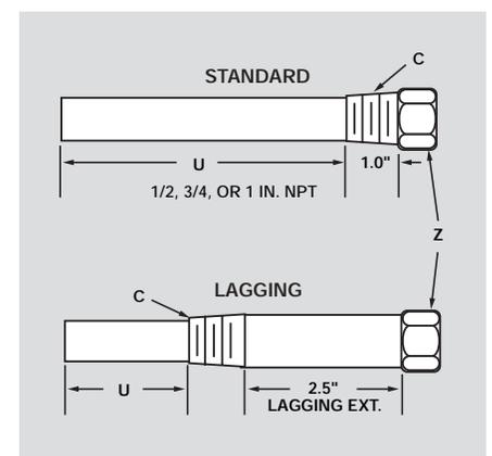
When using P-4 Bulb with a thermowell dimension X + J on thermal system must exceed E dimension of the well plus any lagging extension by 2 inches.
