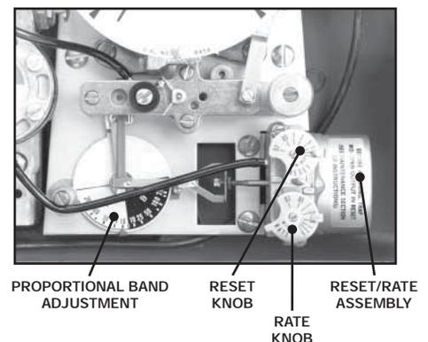
**DIFFERENTIAL GAP ACTION:** This is a two-position control mode standard in all Model 40 Proportional Controllers. The output pressure of the controller remains at maximum (20 psi standard) or minimum (0 psi) until the controlled measurement crosses a band or gap,
