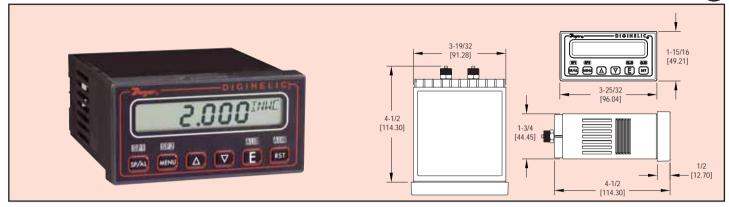
The Series DH Digihelic® Differential Pressure Controller is a 3-in-1 instrument possessing a digital display gage, control relay switches, and a transmitter with current output. Combining these three features allows the reduction of several instruments with one product, saving inventory, installation time and money. The Digihelic® Controller is the ideal instrument for pressure, velocity and flow applications, achieving a 0.5% full scale accuracy on ranges from 5 to 100 in. w.c.
