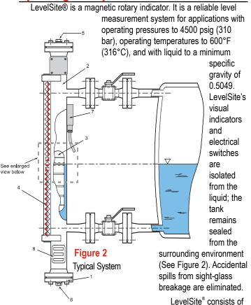
3 major components: the float housing, a magnetic float, and the rotating flag assembly. The float housing is an engineered pressure vessel which is externally mounted to the tank. The float
