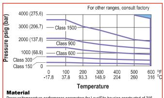
Pressure/temperature performance parameters for LevelSite housing constructed of 316 stainless steel are specified in the chart. Please consult the factory with pressures/temperatures requiring other alloys.
