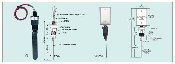
V8 Flotect<sup>®</sup> Flow Switch Protects Equipment: Operation is simple and dependable. In most applications, the switch is normally off while there is sufficient flow of liquid or air. When flow stops, the vane spring moves the vane, actuating a single pole double throw switch rated 5A @ 120/250 VAC to start or stop motor, pump, engine, etc. Operate a damper or valve; shut down a burner or actuate an alarm or signal, protecting unattended equipment from damage or loss of production.
